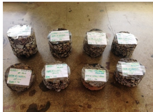
Fig. 5: Road Samples Collected Using Core Cutter
